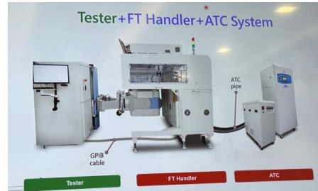
Fig. 172: The ATC is integrated into the handler
