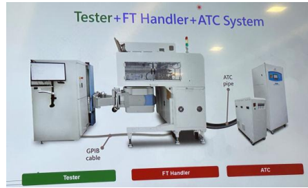
Fig. 248: The ATC is integrated into the handler
