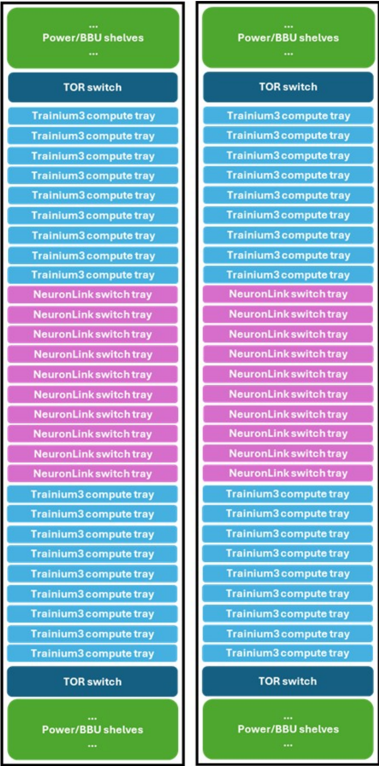
Exhibit 17: AWS Trainium3 UltraServer architecture
