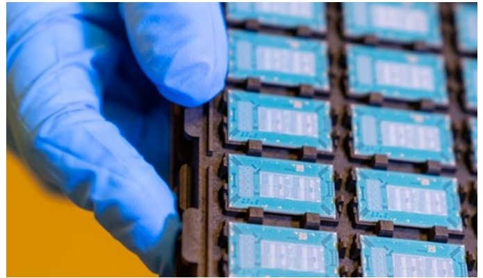
Exhibit 10: Packages with Glass Core Substrates
