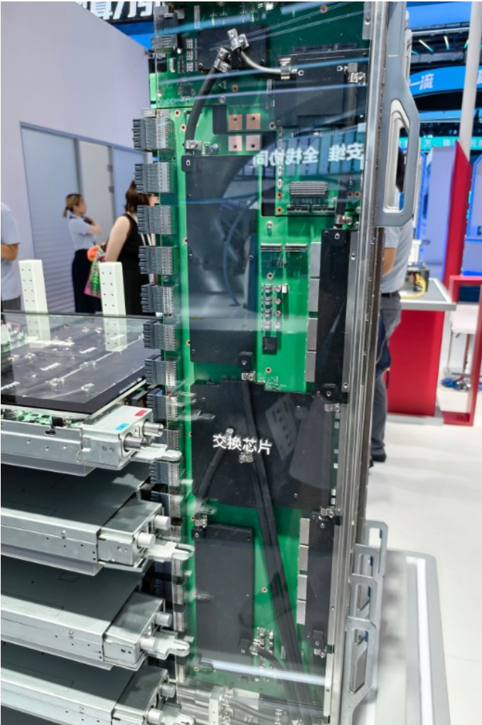
Exhibit 6: Midplane-free orthogonal designs at WAIC
