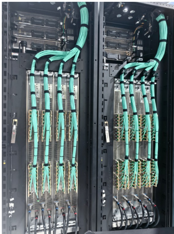
Exhibit 3: The reverse side of Atlas 950 mainly showcases the optical interconnects adopted by ULink
